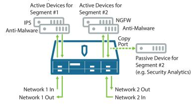
Copy Ports: using a unique "Decrypt Once, Feed Many" design, the SSL Visibility Appliance is capable of sending copies out to many devices over the additional ports on the device. This allows organizations to feed all traffic (decrypted and non-SSL) to additional passive devices on the network.
